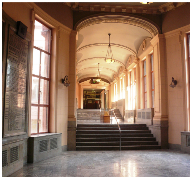
The main elements of fireproofing in the Legislative Library are steel shelving, metal furniture, marble floors, and steel and copper railings. The North Wing is separated from the main building by a long corridor, shown above, with fireproof doors at both ends.
